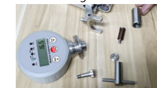
④ Take out the pressure needle and replace it with a new needle
